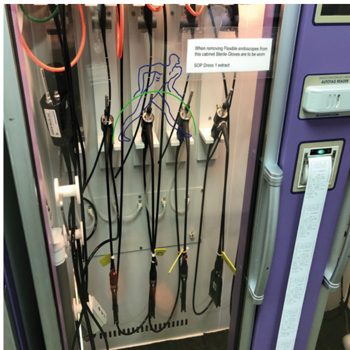
Endoscopes fitted with passive RFID tags
